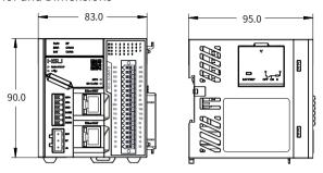
Figure 3 Exterior and dimensions (mm) of the PLC
